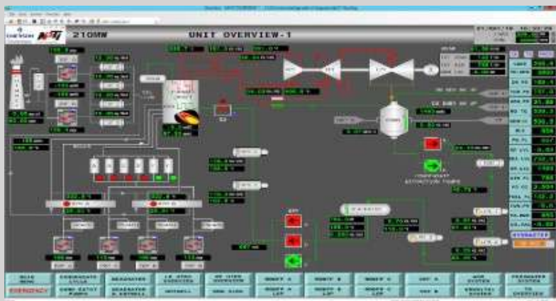
210 MW Sub-critical Simulator
